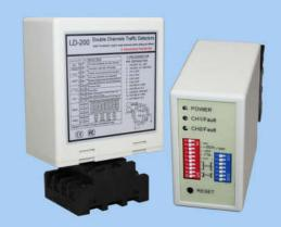
The loop is part of an oscillator circuit. The oscillator is held just on the verge of oscillation via AGC. When a car enters the loop it "dampens" the loop by absorbing energy, and the oscillation decreases or stops entirely. The circuit needs a very long time constant in the AGC loop in order to detect slowly moving
