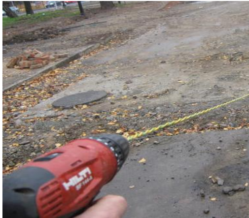
Fig.9. - Method of twisted pair multiwire cable 1,5-2,5 (mm 2 ) copper (at least 10 twists per meter) [1]
